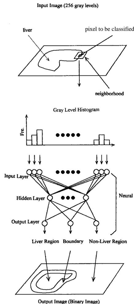
**Fig. 2** Schematic diagram of our boundary detection method using a neural network.
