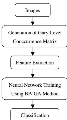
**Fig. 3** Block diagram of classification scheme.
